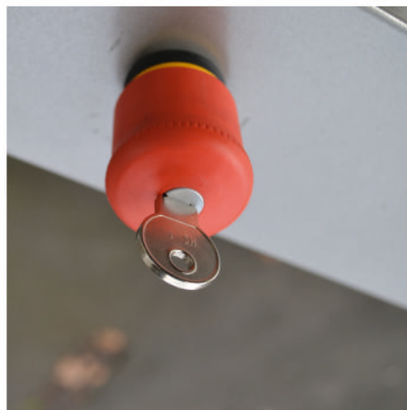
Emergency stop button, lockable.
